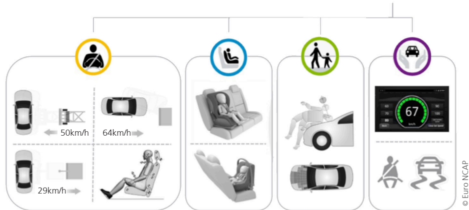
Picture 1. Four areas of Euro NCAP post-2009 protocol assessment: car occupant protection, child occupant protection, pedestrian protection and safety assist.
